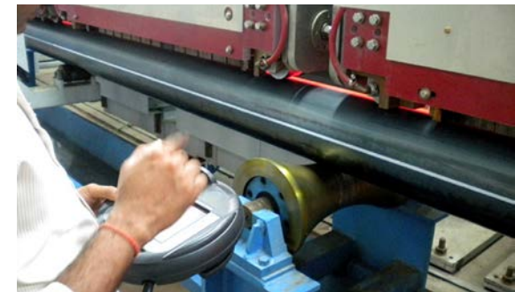
The control system helps meet the challenges posed when normalizing weld seams on the new generation of API-standard pipe.
