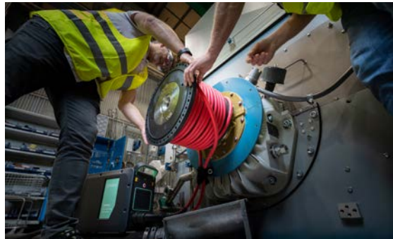
Ventac air-cooled induction heating system is ideal for shrink-fitting applications.
