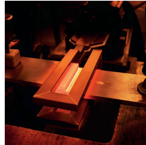
Brazing with an ENRX system. Note how the heating zone is fully visible, something that is practically impossible with flame brazing.
