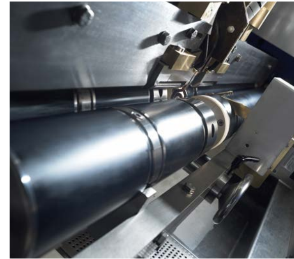
A shaft moving at high speed through an induction coil. Induction tempering is unrivalled for its speed and precision.
