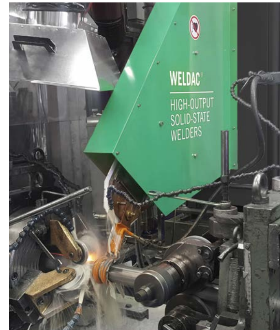
Weldac can be fitted with various induction coils that are very easy to change.
