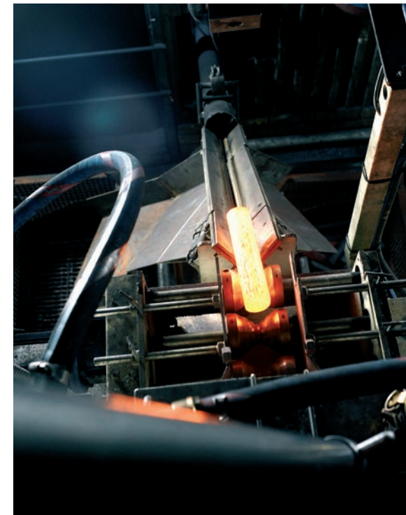
An ENRX vertical partial heater. These systems can be fitted with any number of induction coils, and are available in IGBT and thyristor versions.
