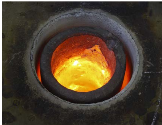
Molten brass in a moving-coil melting furnace. The prefabricated (clay graphite) crucible remains static during the full melting cycle. Instead, the coil moves around the crucible without touching it. Dedicated crucibles – which also act as pouring ladles – eliminate inter-alloy contamination.
