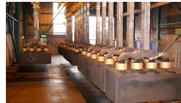
No dust, no fumes, no noise. An ENRX heater gets to grips with 170 millimetre anode stubs.
