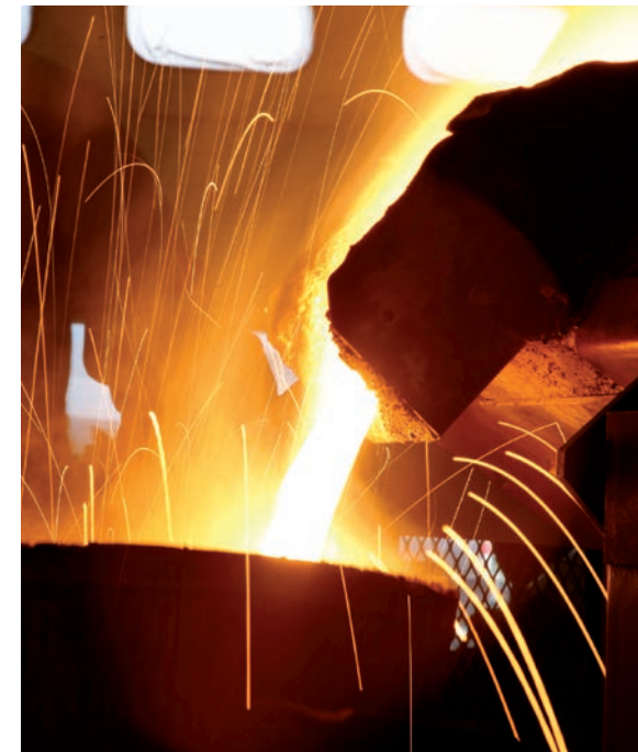
An ENRX single-axis tilt-pour furnace. Such systems can melt ferrous and non-ferrous metals (copper and aluminum alloys). Several models are available to suit all capacity needs. They are available with easy-to-change pre-fabricated crucibles or rammed linings.
