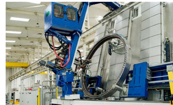
An ENRX solution is used to harden the giant slewing rings used in wind turbines.
